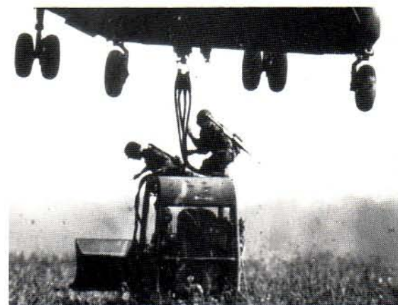
TIME-SAVER — The U.S. Army's new CH-47D Chinook's ability to lift heavier loads than its predecessors allows heavy equipment to be carried intact, thereby avoiding costly disassembly and reassembly time.
